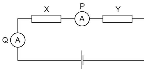
Which ammeter shows the current in resistor Y?
